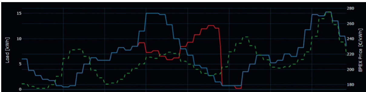
Figure 4: Concept of shifting load profile from evening to night and early morning based on energy prices
